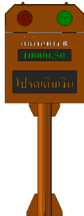
Fig. 1 User Fare Display (Toll Information Point), Typical configuration for Manual Toll Collection
